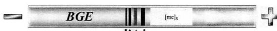
Fig. 2. Schematic diagram of a stacking mechanism by sweeping using a cationic surfactant (with sample matrix containing phosphate buffer).
